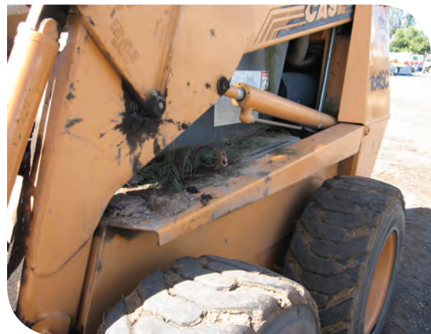
Plant material attached to bobcat.
