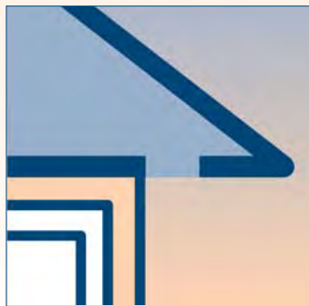
◀ Soffit vent too close to exterior wall
