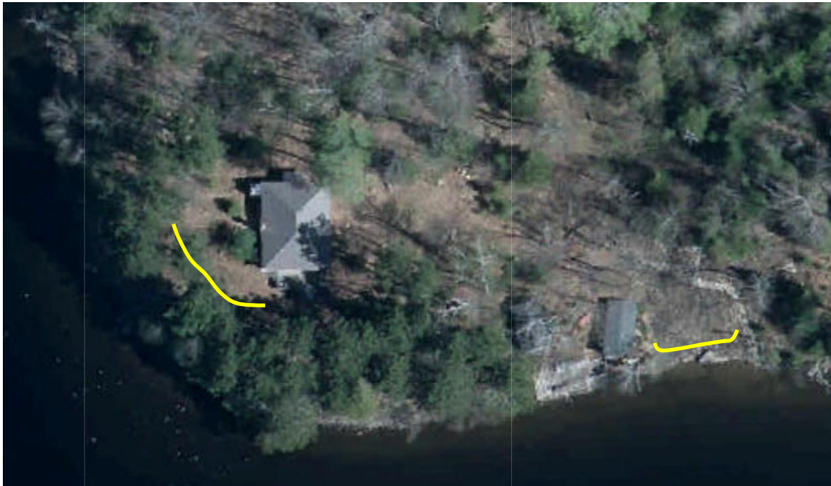
Figure 16 - Approximate location of sediment control barrier(s) (yellow) to be installed between construction area and slope to Aylen Lake, and along the shoreline in the south-east clearing (as needed) (image courtesy CLUPA)
